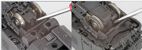
Figure 7: Levering off the gear box cover
